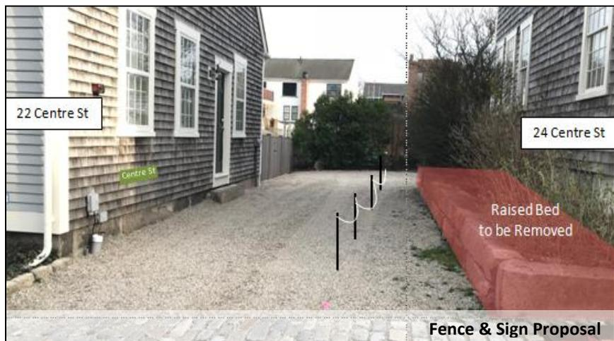
driveway width of 10', a traditional fence would not be functional, therefore the installation of 42" high wrought iron posts and nautical rope to serve as a barrier along the entirety of the west property line is proposed. There will be 11 iron posts, with the first post to be located in alignment with the front façade of the two buildings. A small 4" X 18" painted parking sign is to be attached on the west façade of the building, approximately 24" above grade, below the northwest window.
